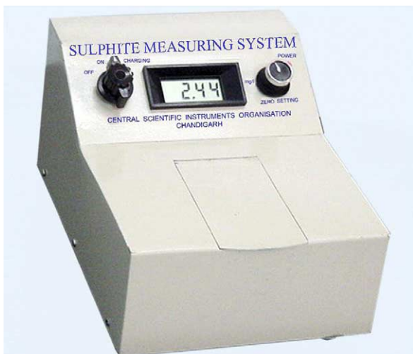
Fig. 1. Optoelectronic instrument for the determination of sulphite.
